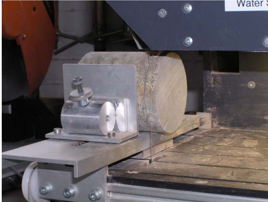
Figure 2 Preparation of the 8-10 mm slices by dry cutting with a diamond wire saw
