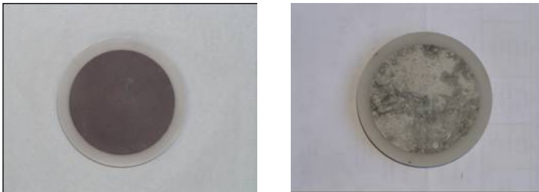
Figure 3 Red shale (left) and limestone (right) samples embedded in epoxy resin
