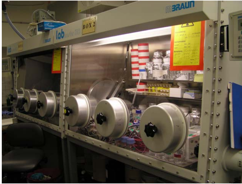
Figure 5 Inert gas glove box in the controlled area of the hotlab facility at PSI
