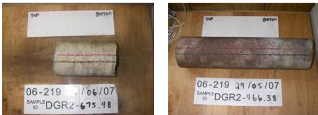
Figure 1 Samples from the deep borehole DGR2 used in the through-diffusion measurements (limestone: left; red shale: right)
